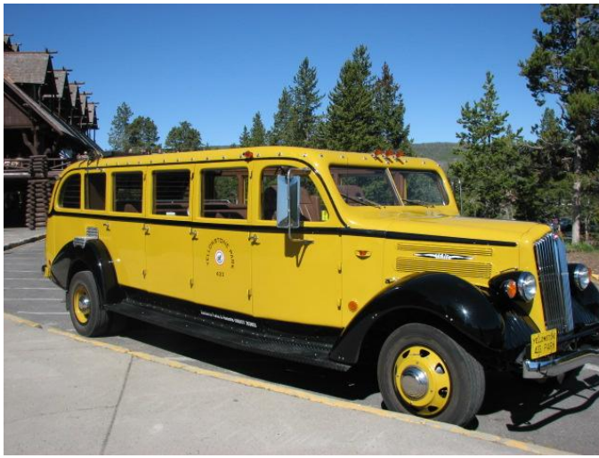
Photo: 20 - A replica of the 1937 bus with a Ford V-8 engine and hydraulic brakes. These are currently used in many National Parks. Photo by Russ Sherwin
