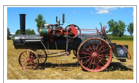
Photo: 8 - A steam tractor, early 1900s from which power could be taken to drive other machinery, like threshers.
