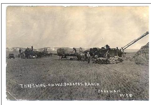
Photo: 2 - Steam tractor driving a threshing machine, late 1800s.
